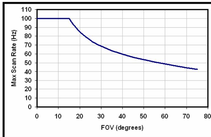
The scan rate is user-selectable from 0 to 100 Hz in 0.1 Hz increments via the graphical user interface. System control software prevents out-of-range inputs for scan rate based on user selection for FOV.
